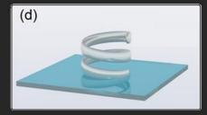
Structure is directly written by moving sample in regard to the focal point
