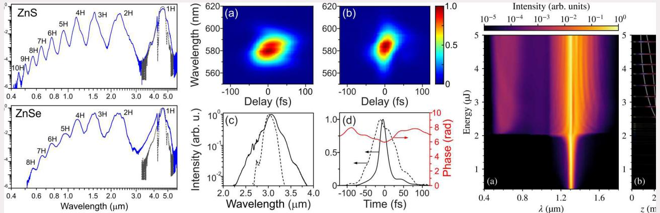
From left to right: harmonics spectra in polycrystalline ZnS and ZnSe excited by 100 fs, 4.6  $\mu\text{m}$  laser pulses; self-compression of 70 fs pulses at 3  $\mu\text{m}$  in a YAG plate making use of anomalous GVD; experimentally measured dynamics of supercontinuum generation and filament-induced luminescence in sapphire.
